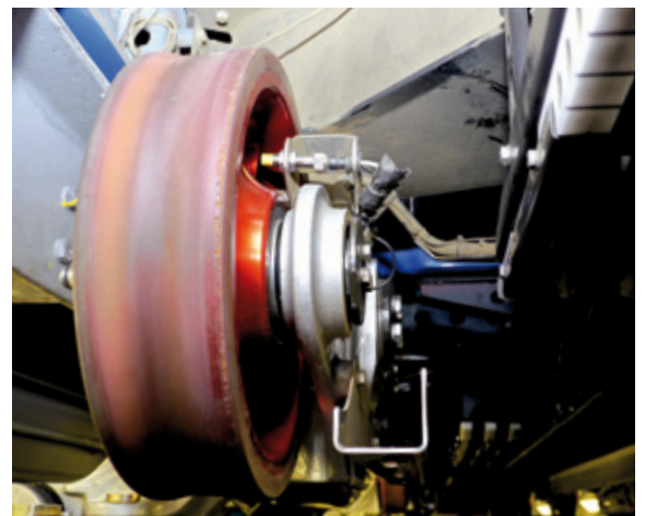
The hole in the alloy wheel of the Megacoaster is detected by the uprox+ with its precise switch point
